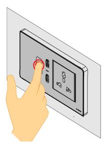
5. After installation, switch on the main electrical power supply and verify that the touch switch is working correctly.
