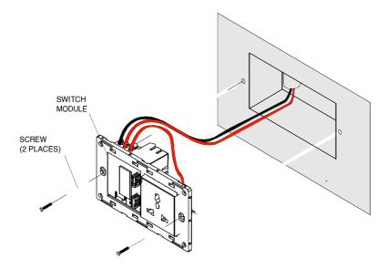
3. Align and position the front touch panel (face plate) onto the switch module.
